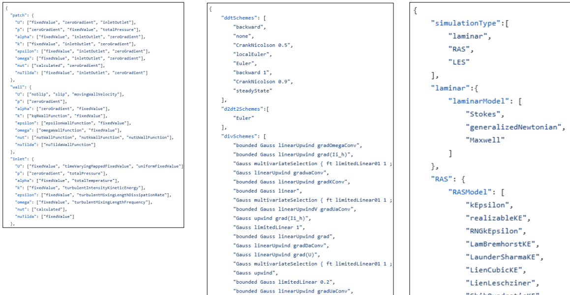
Figure 3: (Left) Directory of boundaryFields comparing setup in blockMeshDict with type choices for each flow variable (Middle) Directory of finite volume numerical schemes that can be used for different mathematical operators in OpenFOAM (Right) Directory of keywords needed to define the turbulence properties
